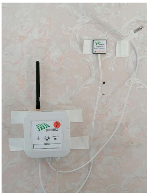
Figure 16: In-situ U-value measurement kit installed on the internal face of a wall (note that the presence of wallpapers may distort the reading)
